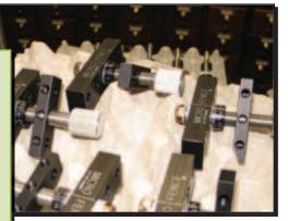
The heart of the Micro Fence system is a micrometer device that allows for precise, fine fence adjustments.
