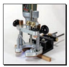
The latest product in the Micro Fence line is this base designed for tools like the Dremel rotary tool, offering fine precision on a smaller scale than standard routers.
