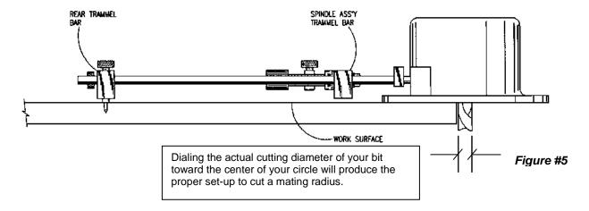
Making circles under 6" diameter with the Micro Fence Circle Jig is a potentially dangerous procedure. Our Center Bar and Leveler Kit, used with our Edge Guide, will allow you to cut diameters as small as one-half inch.
