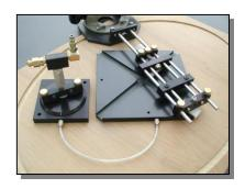
Our Vacuum Center Assembly (VCA) can be used as a remote generator to hold the Standard Ellipse Plate (new version) in position.\* The kit comes with a machined aluminum platform for the VCA, two Parker Mini-loc connectors, 6 feet of vacuum tubing, and the necessary gaskets you'll need to convert your Ellipse Jig to a vacuum hold-down.
