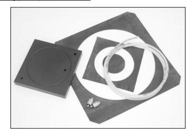
\*On the bottom of the aluminum vacuum block, you will see a 10-32 allen set screw installed that has been wrapped with teflon tape. This "plug" can be removed and the 4 ½" gasket can be installed if you wish the remote "pod" to be held down by vacuum as well. (When re-installing the set screw, be sure to re-wrap with the teflon tape).
