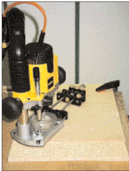
Cutting the outer radius with the Circle Jig
