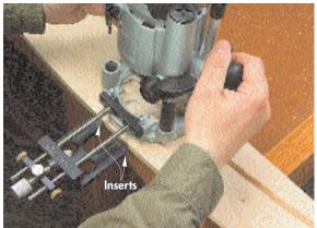
■ The circle jig accessory kit turns the MicroFence into an incredibly accurate circle jig for diameters ranging from 6" to 24".
