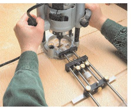
Thanks to its precision adjustment mechanism (Inset), the MicroFence takes the guesswork out of routing perfectly-sized dado joints. It's shown Above with a low-profile fence for routing dadoes at exact intervals.
