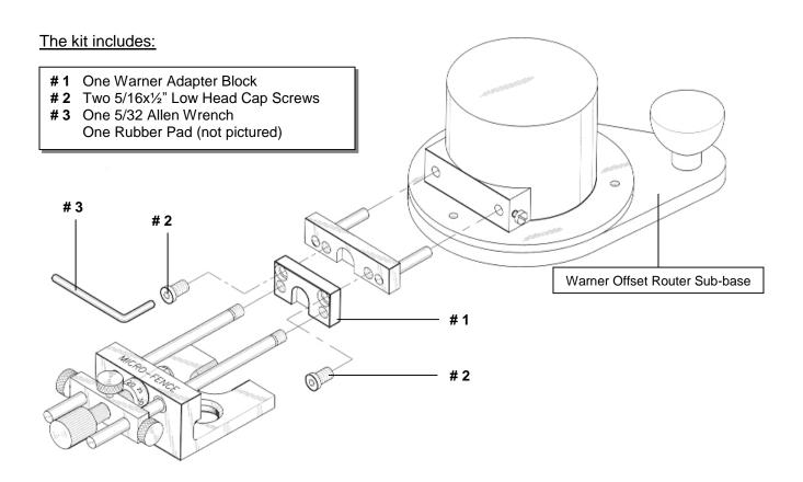
Remove the 7 or 12" guide shafts using the rubber pad, (and pliers if necessary), being careful not to scratch them. Install the block (#1) as shown in the exploded drawing above, and then re-install the stainless rods in the lower-positioned holes. This assembly will provide enough vertical clearance for the body of the Micro Fence to slide under the thicker sub-base.
