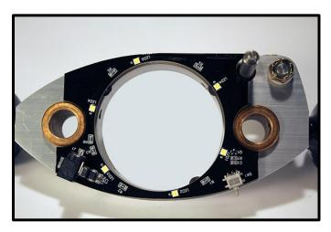
Take care to position the circuit board to provide clearance for the Stop Rod to operate.
