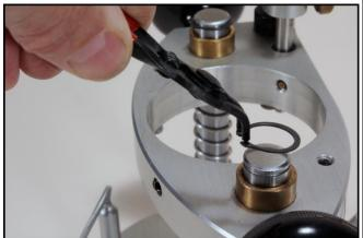
2. When both snap rings have been removed, the motor carriage and plunge springs can be removed. This will permit thorough cleaning of both the chrome posts and the inside of the bronze bushings with DynaGlide Plus.
