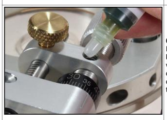
6. Though infrequently needed, a single drop of Phil Oil applied to the micrometer spindle will keep it operating smoothly. (Note: Excessive oil will only serve as a dust trap and cause a build-up of dirt and grime.) Apply an occasional single drop of Phil Oil under the spindle's locking thumbscrew.
