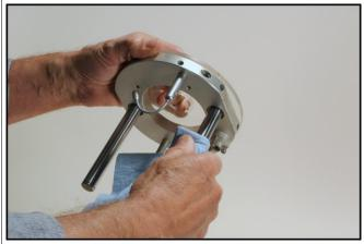
5. Wiping down the chrome posts with a paper or shop towel sprayed with DynaGlide will both clean and distribute the lubricant for complete coverage.
