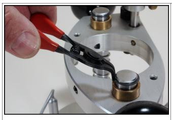
1. When cleaning either of our regular or Micro Plunge Bases, start by removing the external snap rings at the top of the chrome-plated posts. Squeezing the handles of the snap ring pliers together will expand the snap ring so that it can be removed from it's groove..
