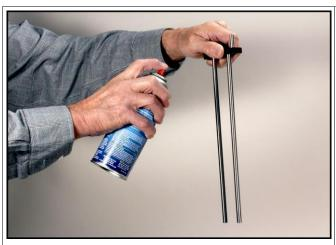
7. On a frequent basis, spray the guide shafts of the Edge Guide and/or Circle Jig with DynaGlide Plus to keep them clean and smooth. If oxidation has occurred, scouring the stainless shafts with #0000 steel wool can bring back their lustre.
