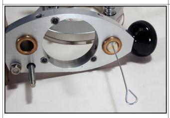
3. Use one of the wool swabs sprayed with DynaGlide Plus to clean the inside surfaces of both bronze bushings. After wiping the swab clean, repeat until no further dirt or grime is seen collecting on the swab.
