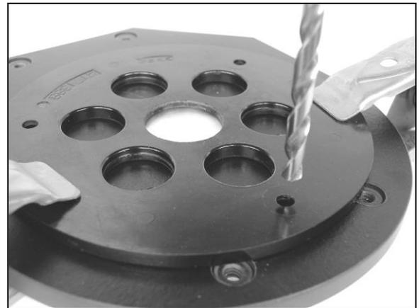
After fastening the router's base to the **Universal Plate**, install the two **Trimmer Posts (#4)** using the 10-32 flat-head phillips screws (**#5**) from the bottom, and fitted with the pan-head screws (**#3**) in the top.
