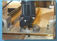
Cleans and prevents router bearing heat build-up to extend bearing life.
