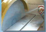
Removes and prevents build-up on abrasives.
